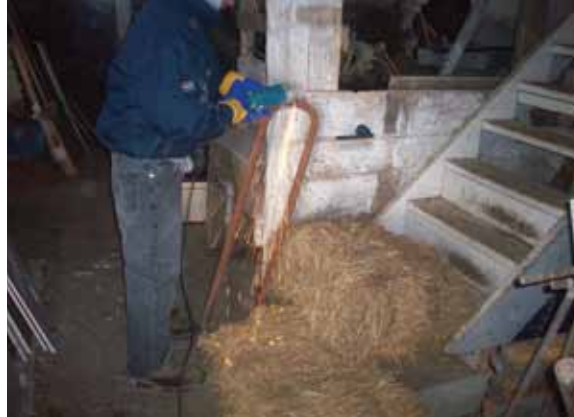
Figure 1.3. Grinding operation taking place in the presence of combustible materials. Use this type of equipment outside the barn and away from combustibles, or put safeguards in place to reduce the risk of accidental ignition.
