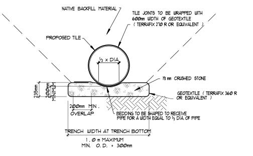
CRUSHED STONE BEDDING DETAIL
